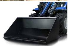
The MultiOne bucket design enables good visibility to the cutting edge, making loading, grading, and dumping more efficient. Length of the bucket has been optimized in order to give best possible breakout force. Heavy duty steel construction includes reinforcement plates inside, slide wear bars on the bottom of the bucket, and the cutting edge is designed for bolt-on teeth.
