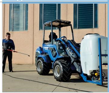
The powerful 170 bar (2,465 psi) pressure jet cleans dirt, built up and dry mud, waxes, oils, grease, strips old paint, and more from any surfaces. This pressure washer system makes cleaning buildings and graffiti removal an efficient process.
